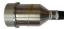
Figure 3: BC-501A (NE-213) and BC-519 liquid scintillators. Cylindrical detection part of thickness 5.08 cm and diameter 12.7 cm. Photomultiplier Hamamatsu model R1250.
