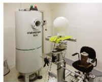
Figure 4: Arrangement of the detector (in the middle), ^{137}\text{Cs} source (on the left) and PuBe source (on the right).
