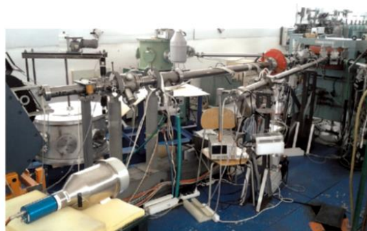
Fig. 5. The experimental arrangement in the Van de Graaff laboratory. The detectors were placed along the beam axis at 1 m distance from the tritium target.
