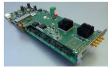
Figure 2: The fast digitizer. The fast digitizer consists of two cards, an ADC card with converters (in the front), and a Combo card (in the back).
