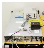
Figure 3: The preamplifier (in the front), the fast digitizer (in the back), and the measuring server (in the bottom).
