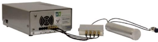
Fig. 1. Two-parametric digital spectrometric system. From the left side: digital spectrometer, amplifier and detector with HV connector.
