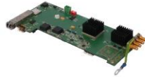
Figure 2: The fast digitizer card. The fast digitizer card consists of AD converter with sampling frequency 1 GHz, FPGA Xilinx Virtex-6 and 10 Gbit optical ethernet.
