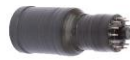
Figure 4: EJ-299-33 plastic scintillator. Cylindrical detection part of thickness 7.62 cm and diameter 7.62 cm. Photomultiplier Hamamatsu model R6233-01.
