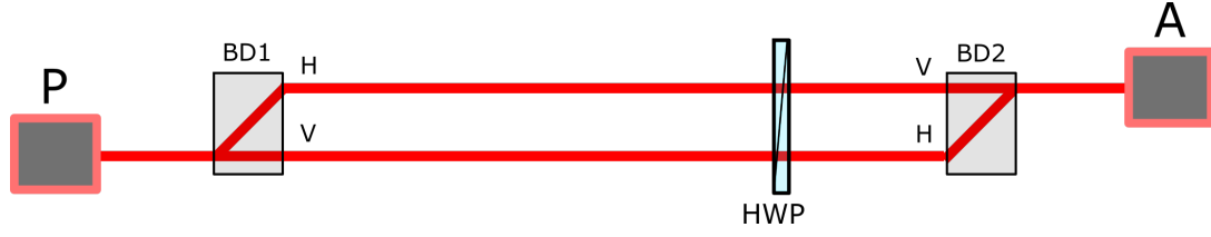
Figure 24: Scheme of the polarization Mach-Zehnder interferometer: beam displacer (BD), half waveplate (HWP), polarization state preparation (P), polarization state analysis (A). The separation between the two paths is 4 mm
