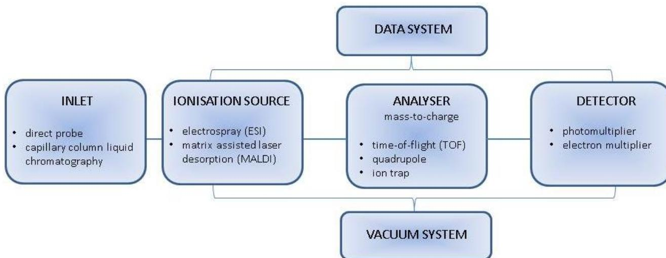
Fig. 4. Simplified scheme of a mass spectrometer with the examples of types in particular components. According to Kinter and Sherman, 2000.
