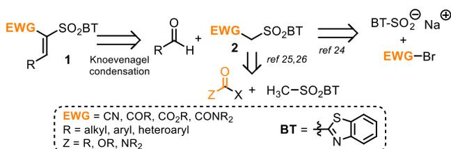
**Figure 2.** Retrosynthesis of trisubstituted vinyl sulfone 1.
