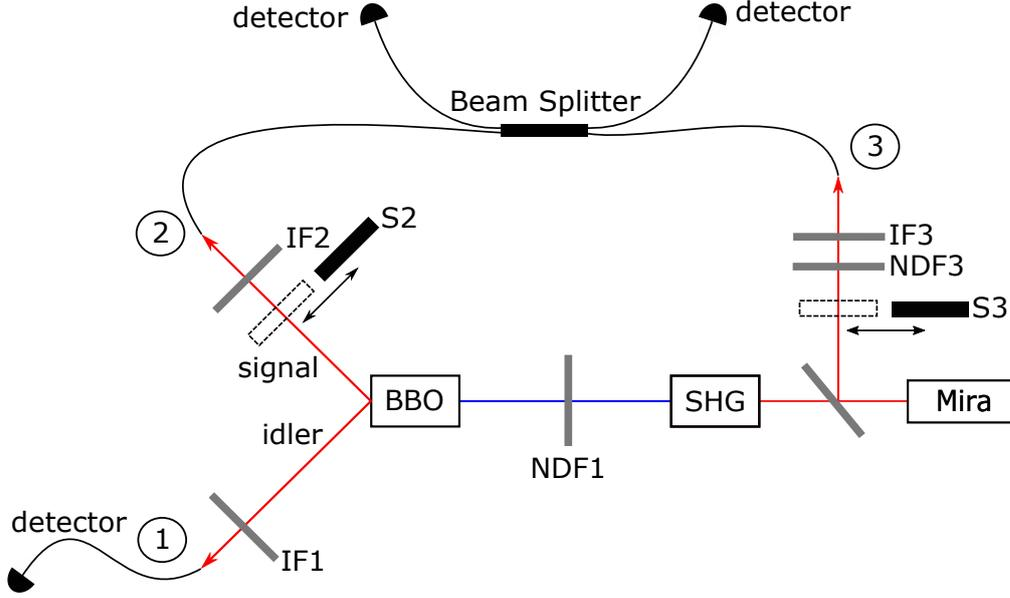
Figure 4.1: Setup of the experiment, 1 – idler mode, 2 – signal mode, 3 – attenuated fundamental laser mode, IF(1-3) – interference filters (3 nm in FWHM), NDF(1,3) – neutral density filter, S(2,3) – shutters, SHG – second harmonics generation, Mira – Ti-sapphire fs laser (central wavelength of 826 nm, FWHM of 11 nm), BBO – a  $\beta$ -BaB<sub>2</sub>O<sub>4</sub> crystal for SPDC.
