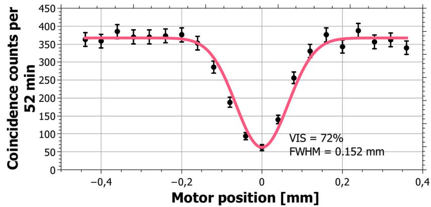
Figure 5.3: Dependence of coincidence counts on motor position. Points visualize experimentally observed results, the solid pink line depicts fitted experimental data with Gaussian function. VIS stands for visibility, FWHM is Full Width at Half Maximum.
