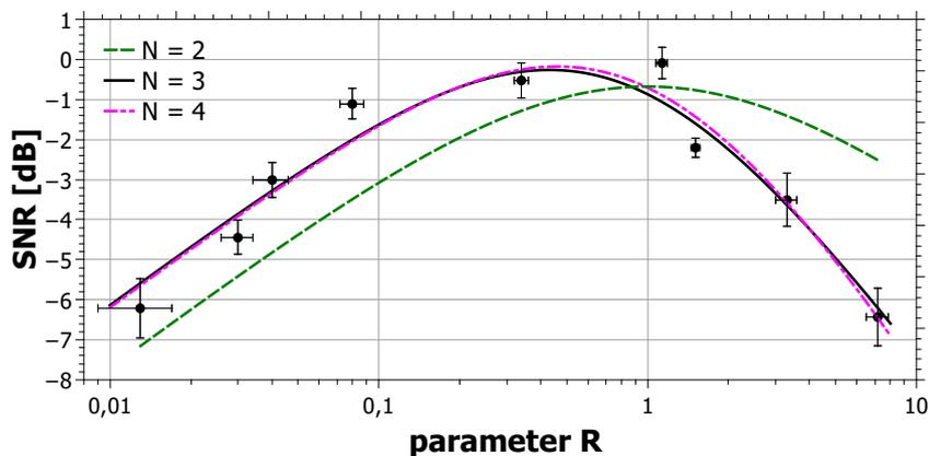
Figure 4.2: Dependence of SNR on parameter  $R$ . Points visualize experimentally observed results. Lines correspond to various levels of expansion in Eq. (3.8): to 2 (green dashed line), 3 (black solid line), 4 (magenta dashed-dot line) terms.
