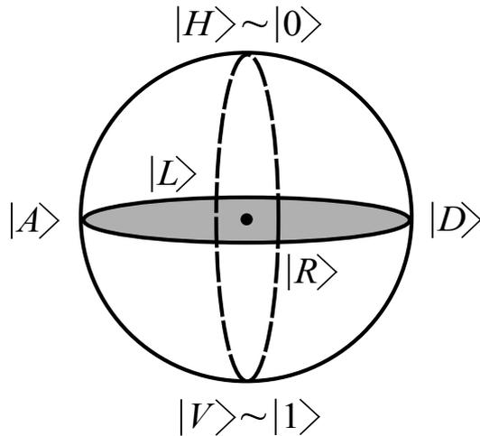
Figure 2.2: Bloch sphere allows easy visualization of polarization states. Polarisation states are labeled as follows:  $|H\rangle$  – horizontal,  $|V\rangle$  – vertical,  $|D\rangle$  – diagonal,  $|A\rangle$  – anti-diagonal,  $|R\rangle$  – right-hand circular,  $|L\rangle$  – left-hand circular.
