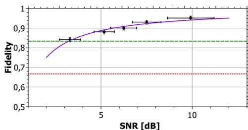
FIG. 5: Dependence of average fidelity ( $F$ ) on SNR. Points visualize calculated results from experimentally observed SNRs. The solid violet line corresponds to our theoretical model, the dotted red line is the classical protocol limit ( $F = 2/3$ ) [32] and the dashed green line indicates the secure teleportation, i.e.,  $F = 5/6$  cloning threshold see [30].
