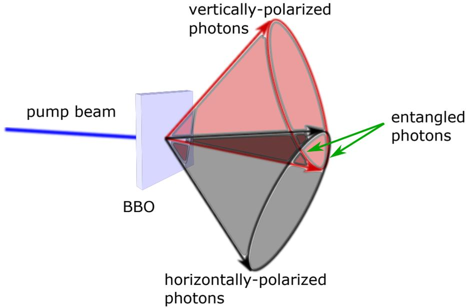
Figure 2.5: The scheme for Type II SPDC process the photons are emitted from the crystal into the surfaces of two cones which can intersect in two, one or zero points. Also the generated photons are entangled in polarization only in the intersections of the cones.
