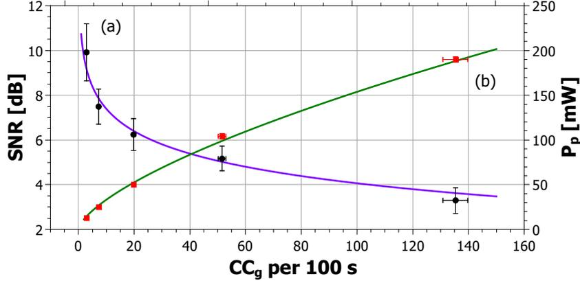
Figure 4.3: (a) Dependence of SNR on genuine coincidence rate  $CC_g$ . Points visualize experimentally observed results, the solid violet line depicts fitted experimental data with theoretical dependence based on Eq. (3.15). (b) Dependence of  $CC_g$  on  $P_p$ . The solid green line depicts fitted experimental data with theoretical dependence based on Eq. (3.9)
