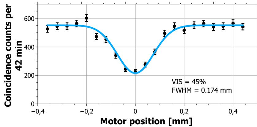
Figure 5.2: Dependence of coincidence counts on motor position. Points visualize experimentally observed results, the solid blue line depicts fitted experimental data with Gaussian function. VIS stands for visibility, FWHM is Full Width at Half Maximum.
