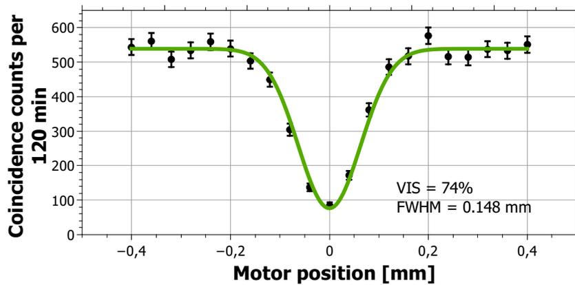
Figure 5.4: Dependence of coincidence counts on motor position. Points visualize experimentally observed results, the solid green line depicts fitted experimental data with Gaussian function. VIS stands for visibility, FWHM is Full Width at Half Maximum.
