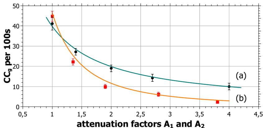
Figure 4.4: (a) Dependence of  $CC_g$  on attenuation factor  $A_1$ . Points visualize experimentally observed results, the solid blue–green line depicts fitted experimental data with theoretical fit based on Eq. (3.16). (b) Dependence of  $CC_g$  on attenuation factor  $A_2$ . The solid orange line depicts fitted experimental data with theoretical dependence based on Eq. (3.16).
