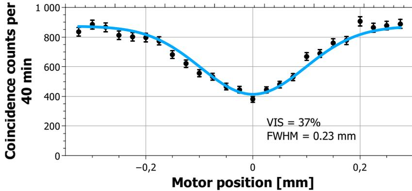
Figure 5.1: Dependence of coincidence counts on motor position. Points visualize experimentally observed results, the solid blue line depicts fitted experimental data with Gaussian function. VIS stands for visibility, FWHM is Full Width at Half Maximum.
