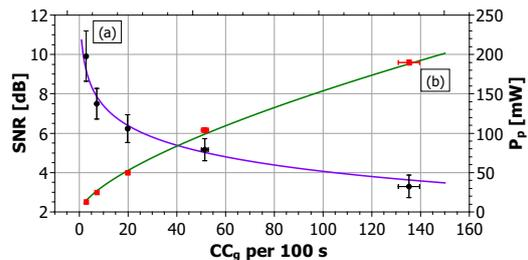
FIG. 3: (a) Dependence of SNR on genuine coincidence rate  $CC_g$ . Points visualize experimentally observed results, the solid violet line depicts fitted experimental data with theoretical dependence based on Eq. (14). (b) Dependence of  $CC_g$  on  $P_p$ . The solid green line depicts fitted experimental data with theoretical dependence based on Eq. (8).
