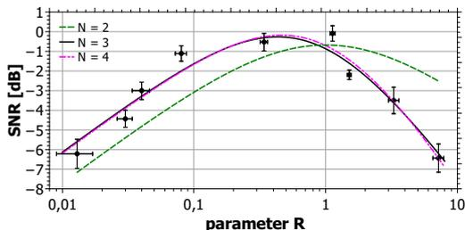
FIG. 2: Dependence of SNR on parameter  $R$ . Points visualize experimentally observed results. Lines correspond to various levels of expansion in Eq. (7): to 2 (green dashed line), 3 (black solid line) and 4 (magenta dashed-dot line) terms.
