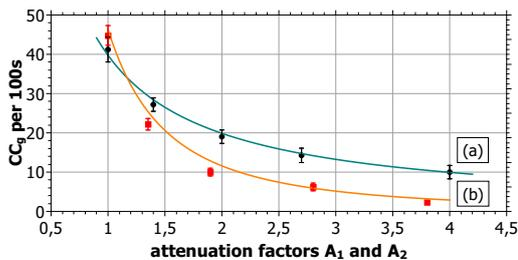
FIG. 4: (a) Dependence of  $CC_g$  on attenuation factor  $A_1$ . Points visualize experimentally observed results, the solid blue-green line depicts fitted experimental data with theoretical fit based on Eq. (15). (b) Dependence of  $CC_g$  on attenuation factor  $A_2$ . The solid orange line depicts fitted experimental data with theoretical dependence based on Eq. (15).
