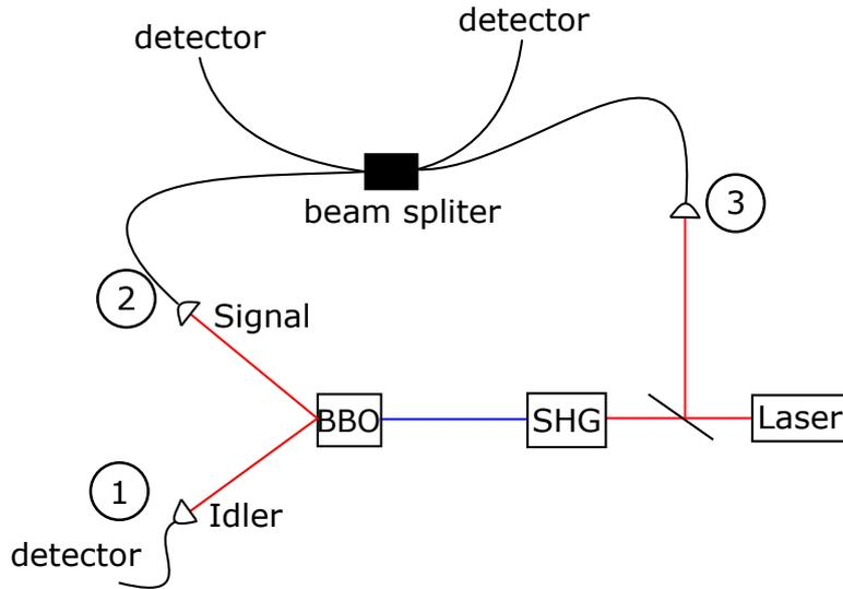
Figure 3.1: Scheme of the experiment, 1 – idler mode, 2 – signal mode, 3 – attenuated fundamental laser mode, SHG – second harmonics generation, Laser – Ti-sapphire fs laser (central wavelength of 826 nm, FWHM of 11 nm), BBO – a  $\beta$ -BaB<sub>2</sub>O<sub>4</sub> crystal for SPDC.
