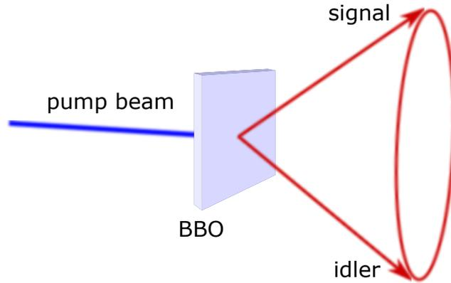
Figure 2.4: The scheme for Type I SPDC process, the generated photons with same frequencies are emitted from the crystal on the opposite sides of the cone surface.
