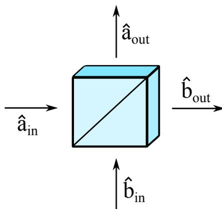
Figure 2.7: The scheme of the beam splitter, that provides the unitary transformation operation on the input modes.
