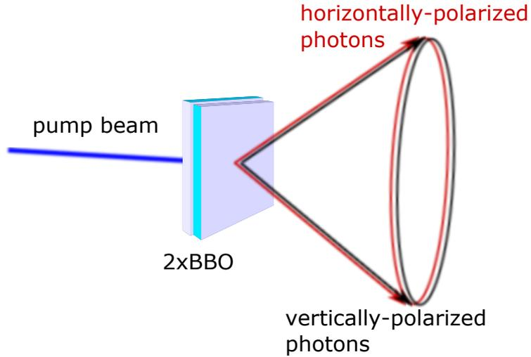
Figure 2.6: The scheme for the Kwiat source of entangled photons.
